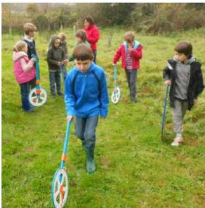
We used trundle wheels and measuring sticks. We measured in cm and metres. The shed was about 60cm. (Noah. C)
